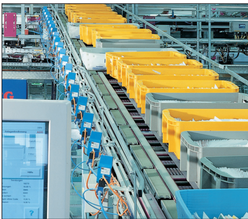
Fig. 3 Checking and triggering accumulation of conveyed objects, as needed
