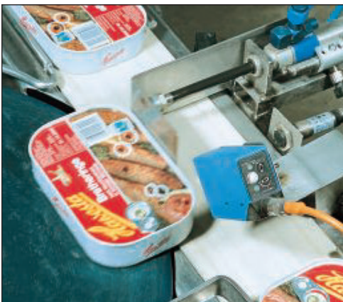
Fig. 4 The CS ensures all cans are packed facing the same way
