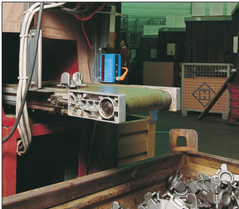
Fig. 4 Counts irregularly shaped objects during production
