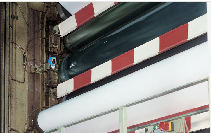
Fig. 7 Monitoring tear off on a paper web
