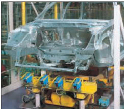
Fig. 4 DME sensor detects drill holes as part of the inspection/quality control process in automotive assembly
