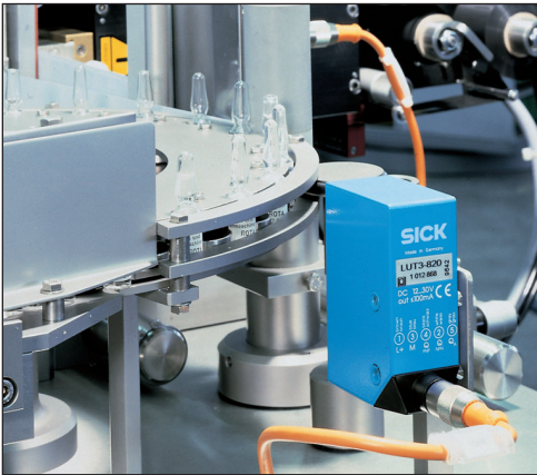
Fig. 3 Label verification by LUT 3-8 in the pharmaceutical industry
