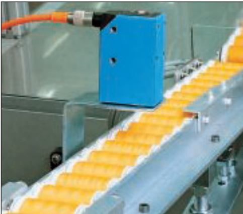
Fig. 3 A CS sensor checking the color of thread before it is packaged
